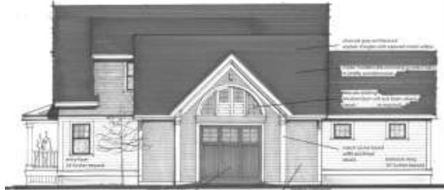
*Presentation Drawing of Carriage House (Barn) Facade at 255 Merriam Street. The existing barn doors and lunette windows are to be carefully removed and reinstalled in the new structure.*
